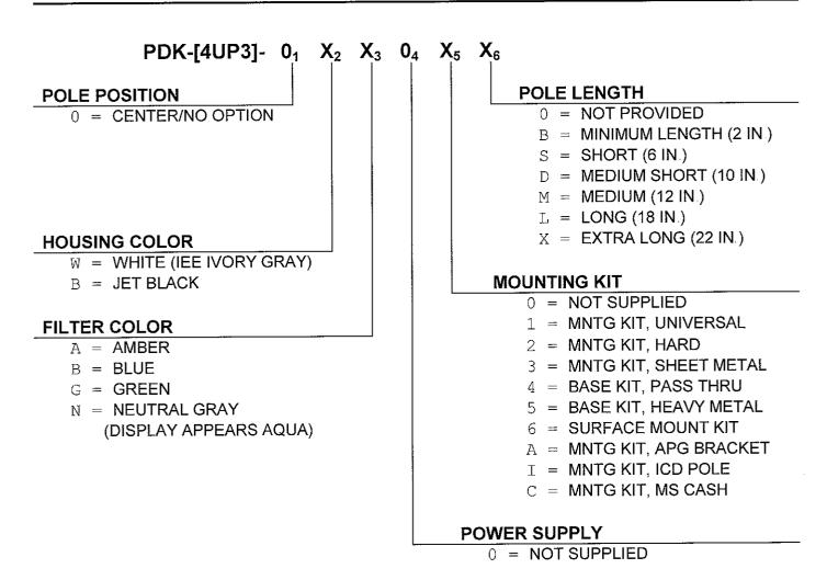
NOTE: THE SUB-SET PDK -[4UP3] -0,1X2X3 DEFINES THE DISPLAY ASSEMBLY IN THIS PDK KIT
